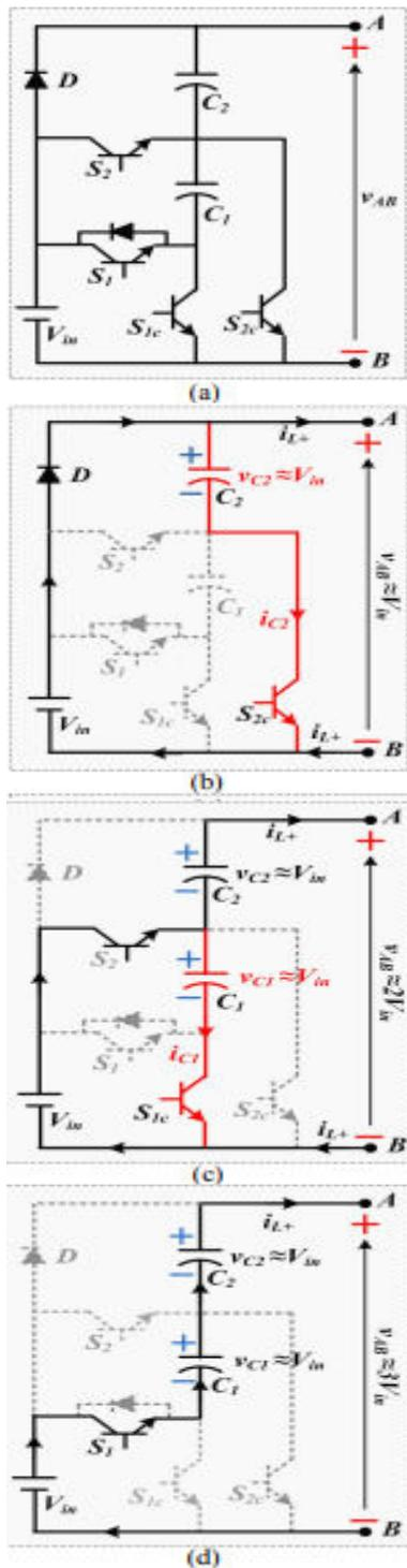
Fig.1. Figure presents (a) BC of proposed SCC; Equivalent circuit and current flow paths of proposed BC when  $v_{AB}$  is (b)  $+V_{in}$ , (c)  $+2V_{in}$  and (d)  $+3V_{in}$
