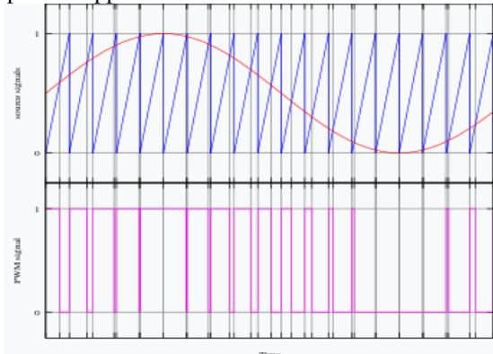
Fig.2: A simple method to generate the PWM pulse train corresponding to a given signal is the interseptive PWM: the signal (here the red sine wave) is compared with a sawtooth waveform (blue). When the latter is less than the former, the PWM signal (magenta) is in high state (1). Otherwise it is in the low state (0).
