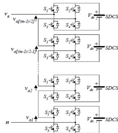
**Fig3:Single-phase structure of a multilevel cascaded H-bridges inverter**
