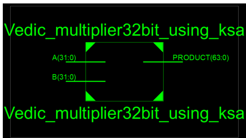
Fig6: RTL Schematic of Vedic multiplier using KSA
