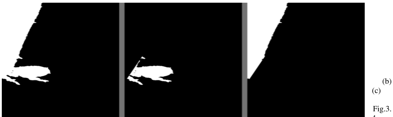
Fig.3.4(b) is obtained by cutting the Fig.3.4(a) with the w-h triangle. The Fig.3.4(c) is obtained by subtracting the (b) from the (a).
