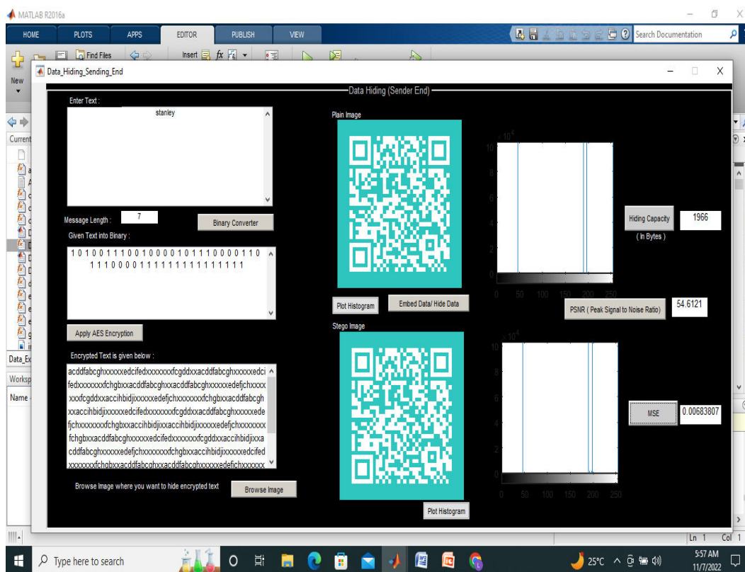
Figure 5 Encryption of message inside a valid qr code
