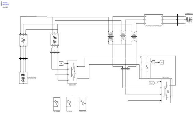
**Fig.3. Simulation circuit.**
