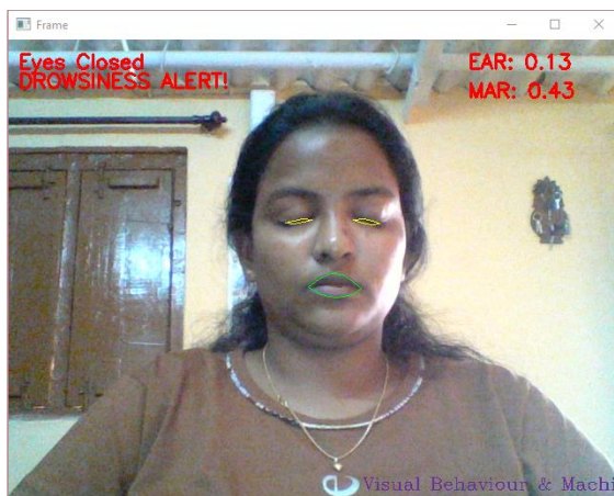
Fig 3,4,5,6 In this real-time test example, an alert sounds if the eyelids are closed for an extended period of time.
