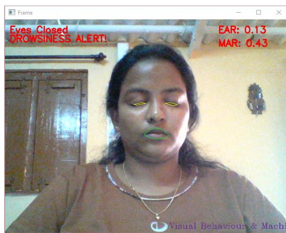
Fig 3,4,5,6 An alarm is sounded when the eyelids are closed for an extended period of time in this real-time test case.
