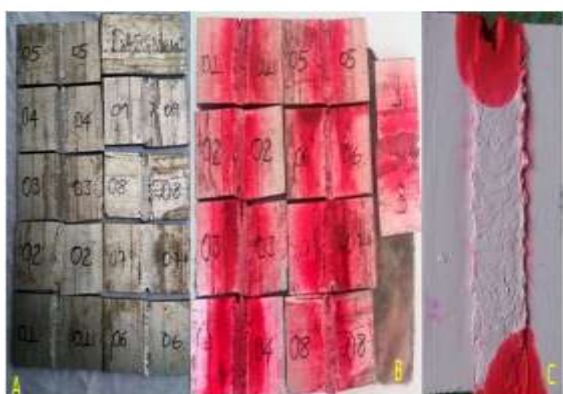
Figure: Liquid penetrant test: (A) Welded specimens before the liquid penetrant test; (B) welded specimens after applying penetrants on the faying surfaces; (C) welded specimens after applying developer.
