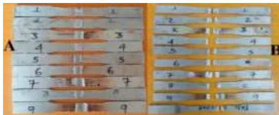
Figure: Extraction of tensile specimens: (A) Welded specimens before the tensile test (B) welded specimens after the tensile test.
