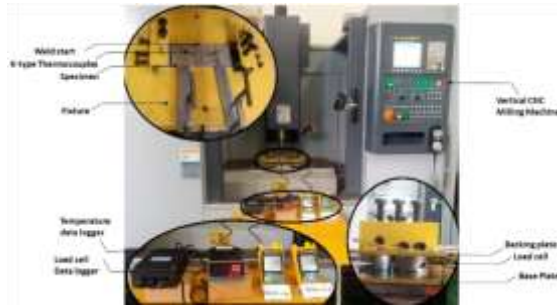
Figure: Experimental setup used for FSW connected with the load cell and thermocouples
