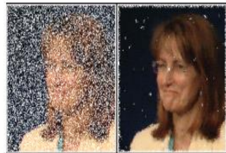
Fig 4: Median filter applied on the image
