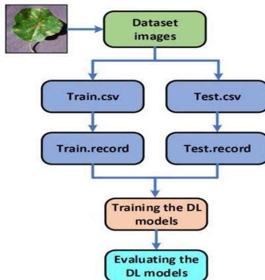
**Fig 2: Generalize framework to train and test the deep learning.**
