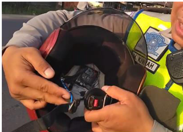
Figure 8. Electronic devices embedded at helmet unit.
