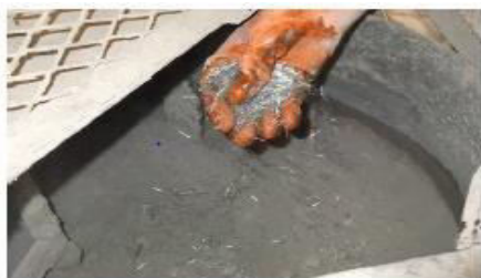
Addition of Fibres to SCC mix
