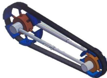
Fig.5 Assembly Design of Hydro-Mechanical CVT
