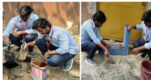
Figure 3 Specimen casting and L – Box test apparatus
