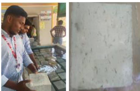
Figure 13 water absorption test
