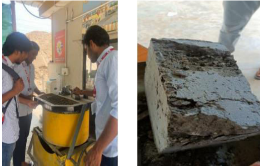
Figure 12 Compression test and tested block
