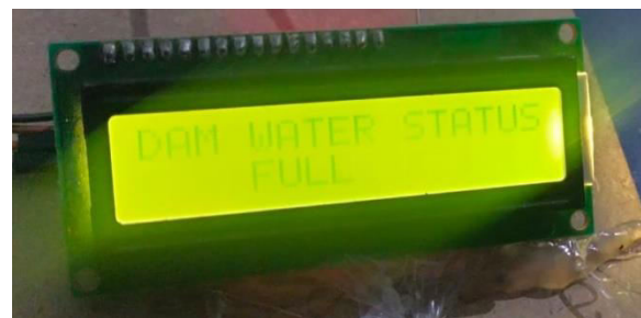
Fig 8: LCD display with water level information DAM full
