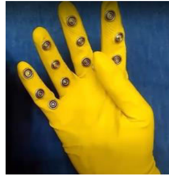
Fig 4: Showing touch buttons integrated with glove
