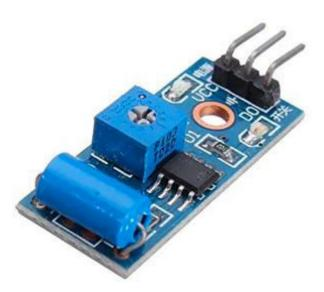
The SW420 Vibration Sensor Module is based on SW-420 Vibration Sensor, which works on the principle that when the movement or vibration occurs, the circuit will be briefly disconnected and output low. Hence the normal state of this sensor is closed. The sensitivity of the SW420 Sensor can be controlled by an onboard potentiometer and LM393 Comparator IC. This is very useful in detecting Collisions, Burglary protection alarm systems, Vibration alert systems, etc.
