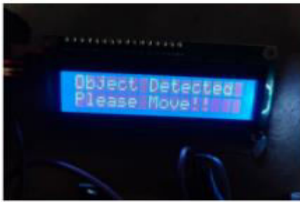
Fig 6.5 LCD Displaying of Obstacle Detection.
