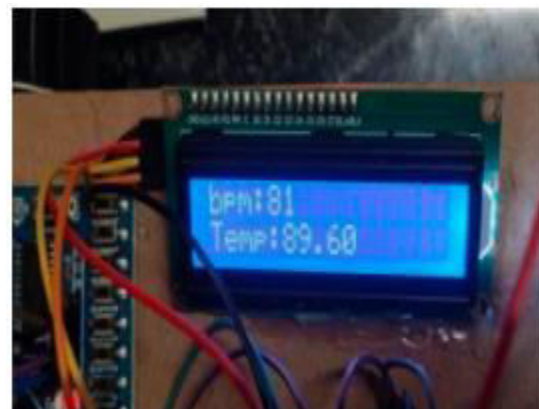
Fig 6.4 LCD Displaying Temperature and Pulse
