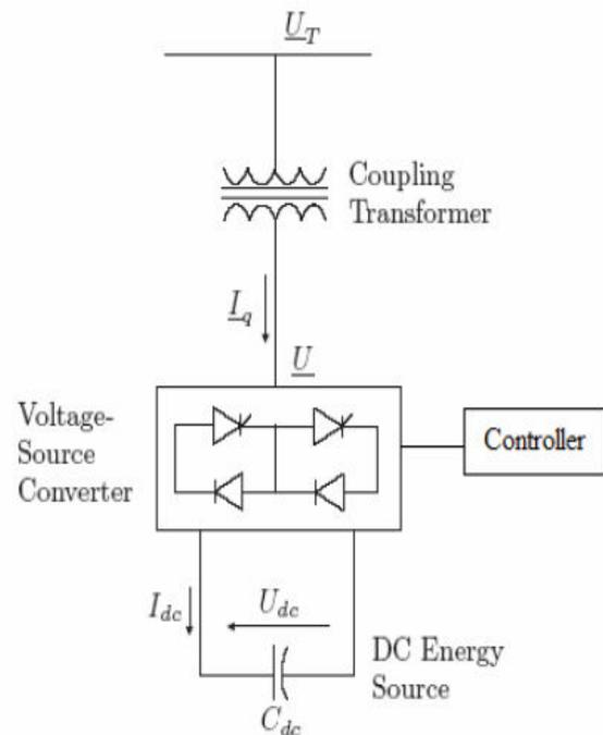
Fig Reactive power generation by a Statcom
