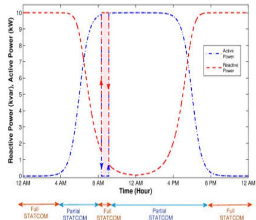
**Fig Concept of smart PV inverter control as STATCOM**
