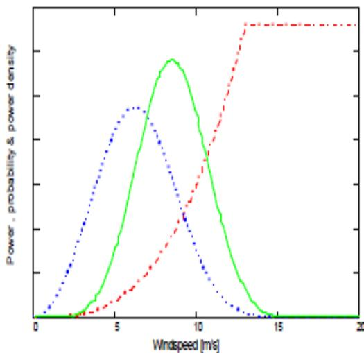
**Fig:** Power P (red, dashed), probability density U (blue, dotted) and power density (green, solid) as a function of wind speed (arbitrary units).
