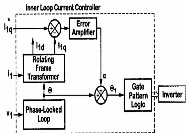
Figure above shows the reactive current control block diagram of the STATCOM. The reference angle,  $\theta$ , is phase-locked to the phase an of the line voltage,  $v_{1a}$ , and is computed using an instantaneous three-phase set of line voltages,  $v_1$ , at BUS 1. Real or direct component  $I_{1d}$  and reactive or quadrature component  $I_{1q}$  are the two components of an instantaneous three-phase
