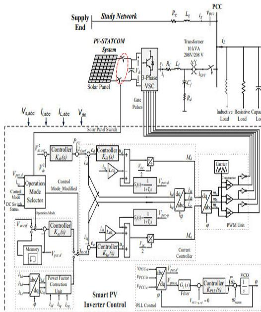
Fig Modeling of the study system and control components
