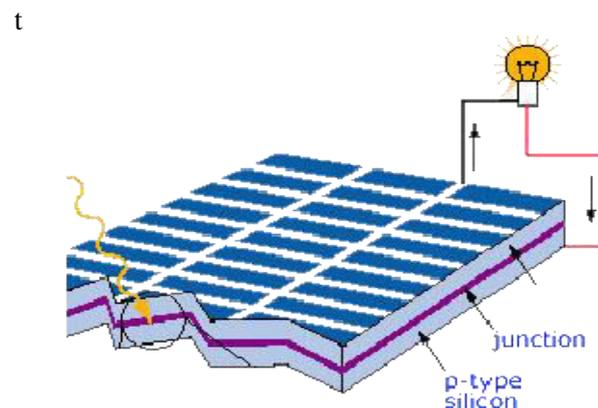
The basic ingredients of PV cells are semiconductor materials, such as silicon. For solar cells, a thin semiconductor wafer creates an electric field, on one side positive and negative on the other. When light energy hits the solar cell, electrons are knocked loose from the atoms in the semiconductor material.
