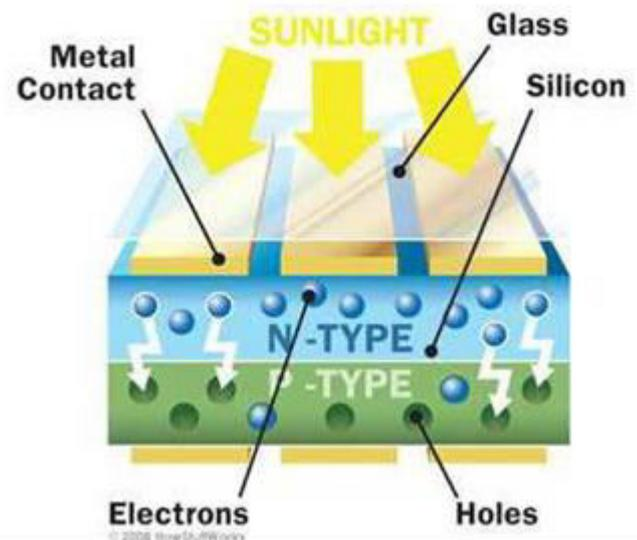
Fig working of PV cell
