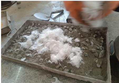
Figure 4 : Adding fibers to the concrete materials
