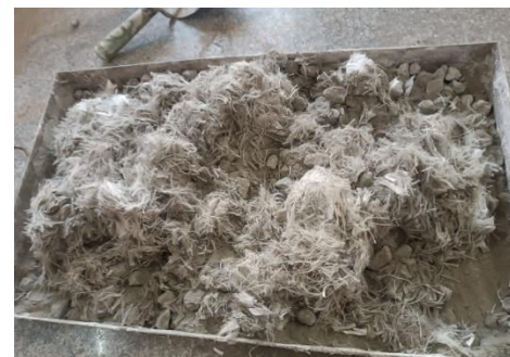
Figure 3 : Mixing of Fibers
