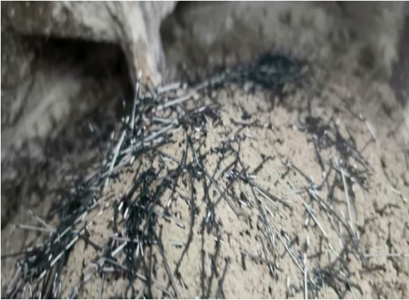
Fig 3.3 Steel Fiber dispersion in GPC
