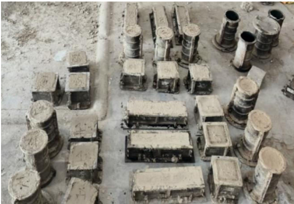
Fig 3.1 Casting of Cubes, Cylinders and Prisms
